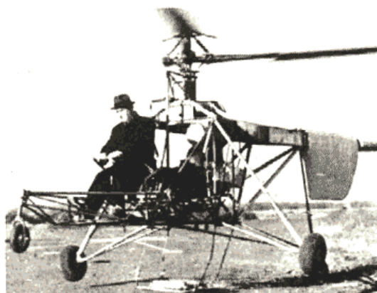
Igor Sikorsky in his VS-300. It used a tail-rotor to stop the airframe from rotating in opposition to the main rotor.
